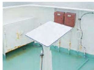
Installation of Starlink Business on vessels (RYUKYU KAIUN KAISHA)
